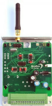
removable chassis and detachable terminal block
